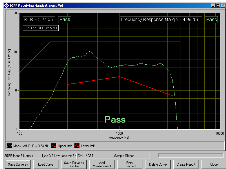
Fig. 29 Receiving frequency response with RLR value displayed
