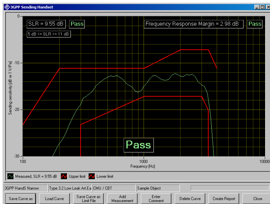
Fig. 28 Sending frequency response with SLR value displayed
