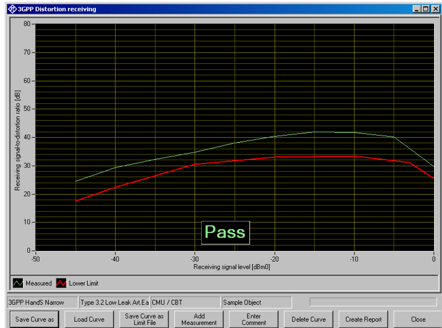
Fig. 34 Typical result of receiving distortion measurement
