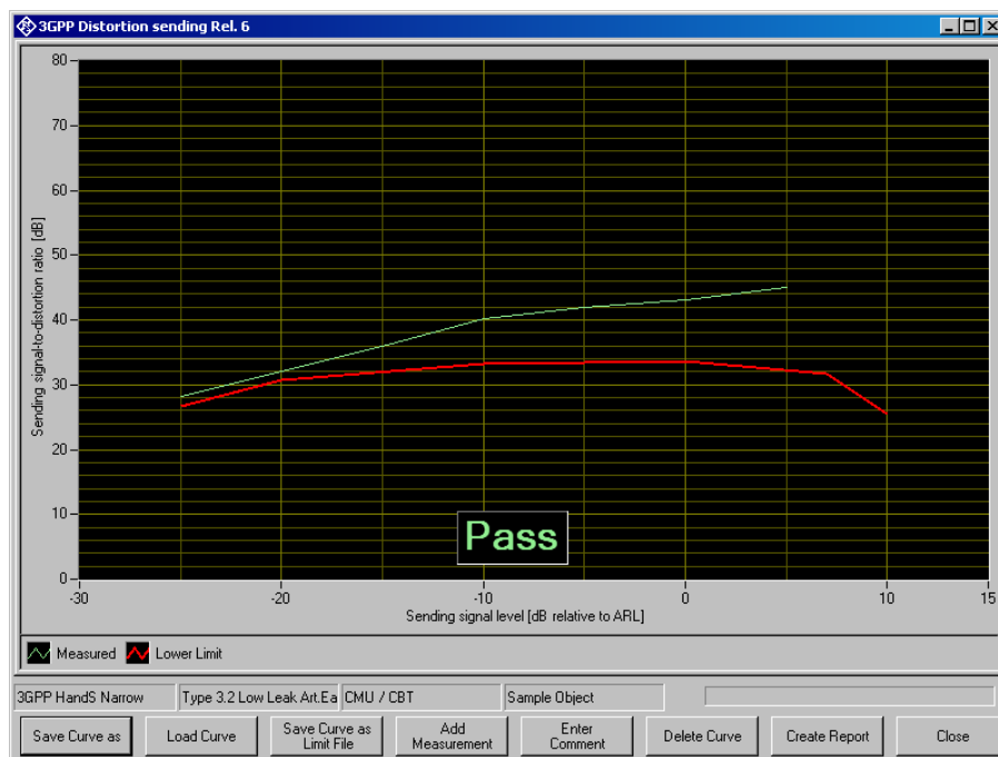
Fig. 33 Sending distortion measurement
